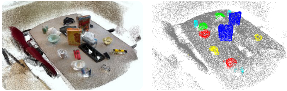
(a) 3D reconstruction of the scene based on a RGB-D sensor. (b) Labeled scene. Each color corresponds to a different object category.
