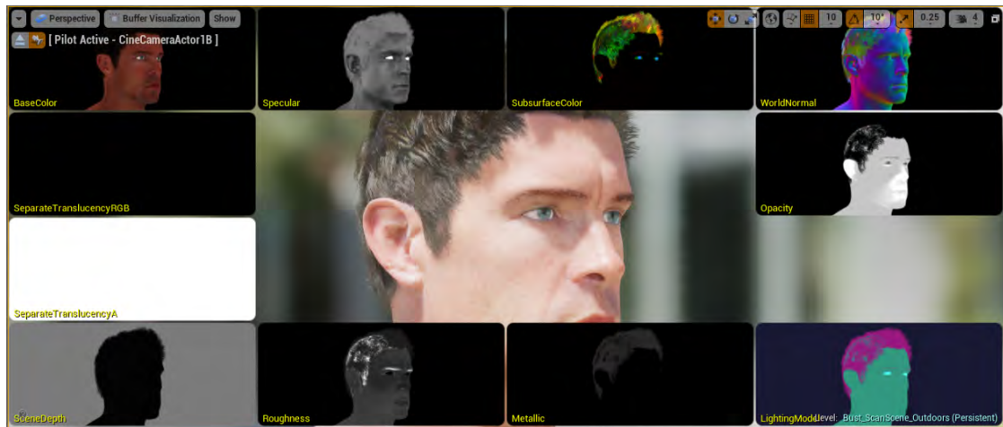
Figure 3.2 The G-Buffer of Unreal’s deferred renderer. Image adapted from [Hof17]
