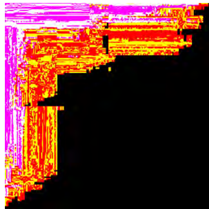
Figure 4.7 Wrong sorting results caused by read-write conflicts during the matrix transpose step.
