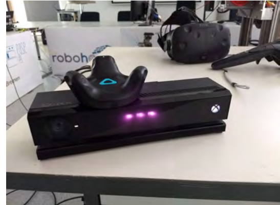
Figure 5.10 The hardware setup for the test: A HTC Vive tracker mounted to a Microsoft Kinect, thus combining Real-Time tracking and 3D scanning.
