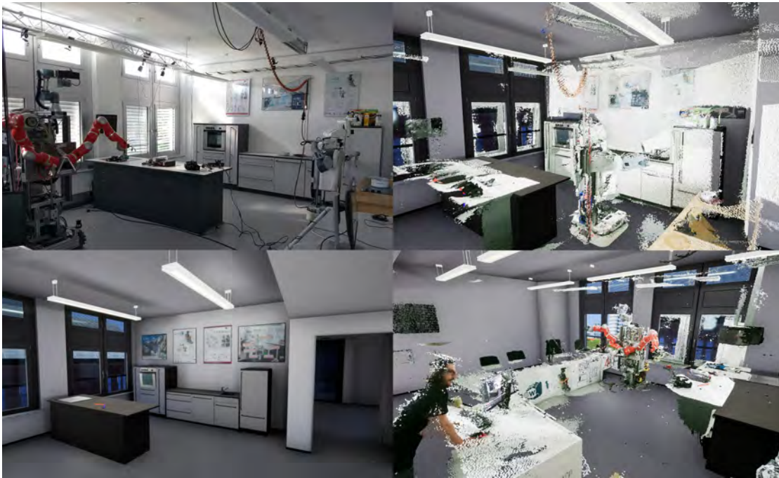
Figure 5.12 The real kitchen testing environment of the Institute of Artificial Intelligence of the University of Bremen (upper left), the precise virtual model of the same environment inside the Unreal Engine (bottom left) and the same environment with additional point cloud snapshots, complementing the virtual representation (right images). One can easily see now that the table in the virtual environment is at the wrong location and not matching with the real-world object.
