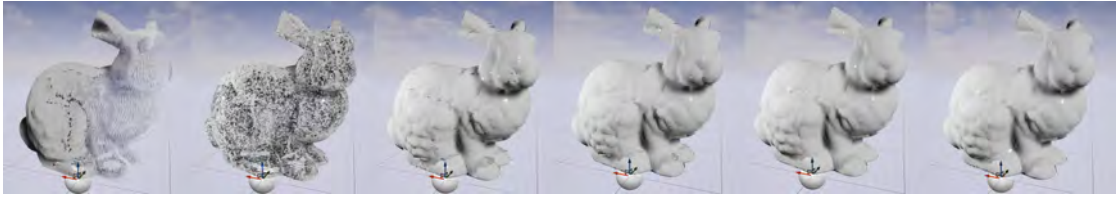
Figure 5.6 The renderings of the bunny dataset by the static point cloud renderer with surface estimation based on k=2, 3, 4, 5, 7 and 11 neighbours (from left to right). It can be seen that for this dataset, a surface estimation based on k=4 yields a reasonable result and that there is almost no visual improvement between k=7 and k=11 .
