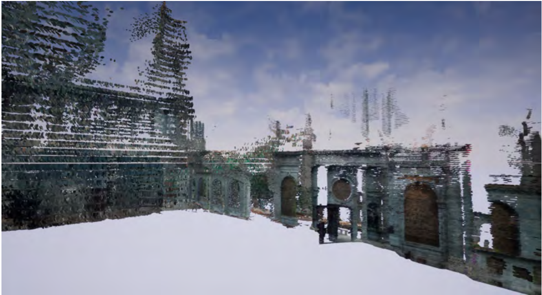
Figure 4.3 Wrong rendering caused by precision loss due to large index helper values.
