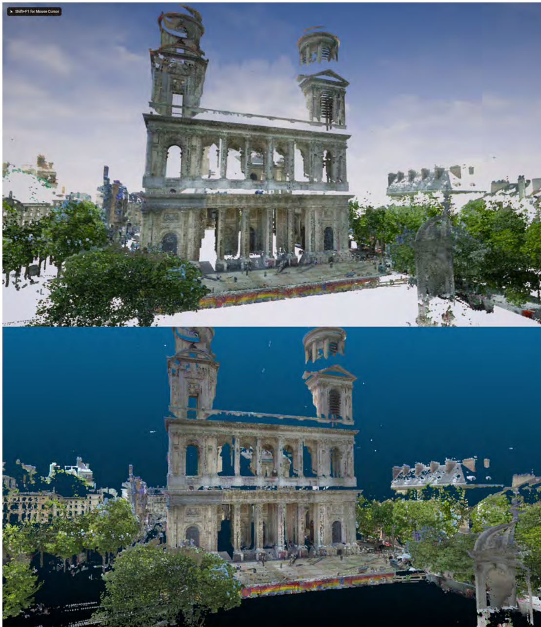
Figure 5.9 The Trimble dataset as rendered by the dynamic point cloud renderer (top image) compared to the rendering by the CloudCompare software (bottom image).
