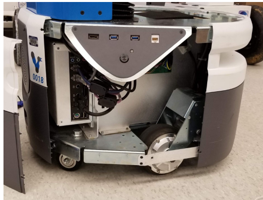
Figure 4.12 A look onto the fetch's differential drive system.
